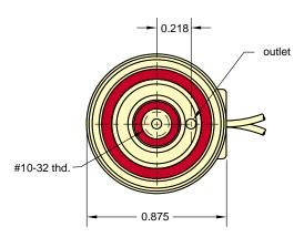
models have two 6-32 threaded, 7/32" deep mounting holes. Manifold models are equipped with a bottom stud, 5/32" long with #10-32 thread, which fits Clippard standard and special manifolds, accessory valves and subplates. Spanner holes in the valve body permit tightening.
